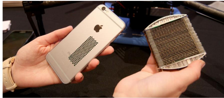
An Apple iPhone and a quadcopter, both retrofitted with hydrogen fuel cell batteries, and a hydrogen fuel cell are displayed by Intelligent Energy at ShowStoppers. Photo by Ann Singer.
